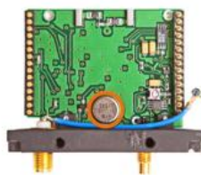
Module providing RF transmission capabilities (other side)
