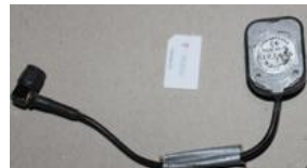
GPS antenna and SIM card
