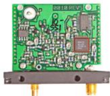
Module providing RF transmission capabilities
