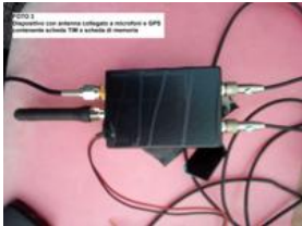
The device with an antenna connected to the microphones and the GPS. It also included a SIM and memory card.
