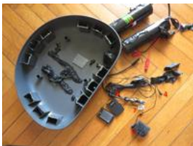
2: the two batteries of the listening device; 4: microphones connected to the listening device; 6: dismantled listening device; 7: SD card.
