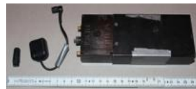
GPS tracker and antenna
