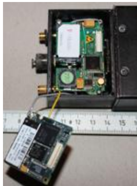
GPS tracker open with SIM card
